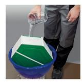
**6.** Prepare any convenient soap solution and apply it with a measuring cup to the workspace (plate stack, core) from all open sides.
