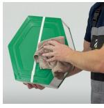
**4.** In case of more severe contamination, in addition to the steps in point 3, add a small amount of cleaner by spraying with a low pressure sprayer (spray gun) or with a measuring vessel on each open side of the working space (plate stack, core).
