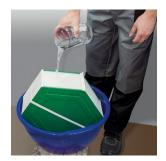
**3.** Apply the disinfectant using a low-pressure sprayer (spray gun) or measuring cup, to each open side of the work area (plate stack, core) and ensure that the disinfectant is distributed over the entire surface. Leave the product for a couple of minutes while the disinfectant will work.
