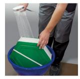
**5.** Place the product back into the cleaned container and rinse the working space (plate stack, core) with running water from all open sides.
