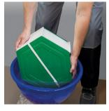
3. For added effect, fill the container with water, dip the product in the water and with smooth reciprocating movements run the water through the core (plate stack) to remove any dust, dirt or other impurities.
